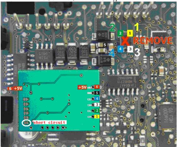
After connection insulate Mercedes CAN filter board with heat shrink or insulation tape. Put it carefully to EZS casing.
