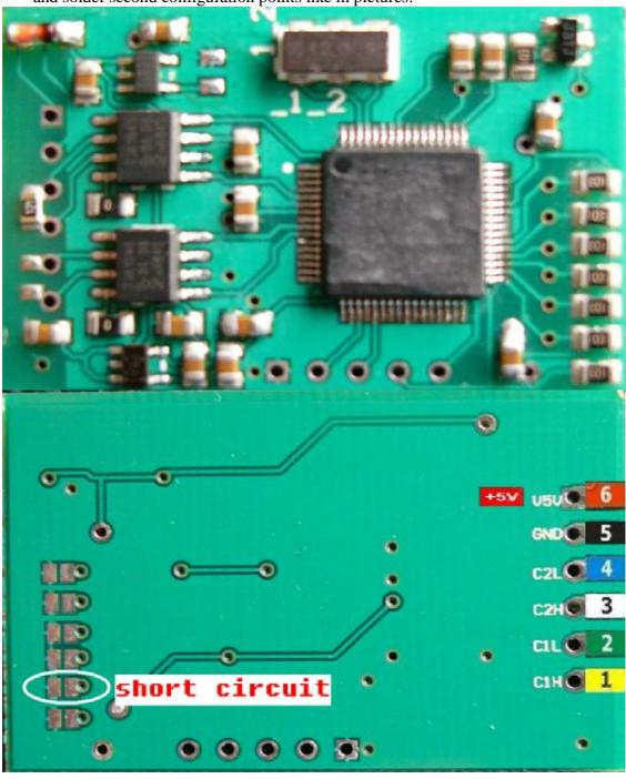
Remove from EZS board SMD part marked with red "X". With short, good isolated wire connect Mercedes CAN filter to EZS board according picture: 1-1 (C1H), 2-2(C1L), 3-3(C2H), 4-4(C2L), 5-5(GND), and 6-6 (+5V).
