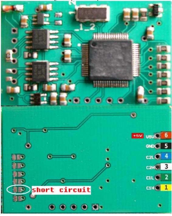
Remove EZS board from casing. Carefully disconnect board from mechanic – look on picture.
