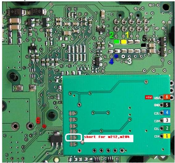
Remove from EZS board SMD part marked with red "X". With short, good isolated wire connect Mercedes CAN filter to EZS board according picture: 1-1 (C1H), 2-2(C1L), 3-3(C2H), 4-4(C2L), 5-5(GND), and 6-6 (+5V).
