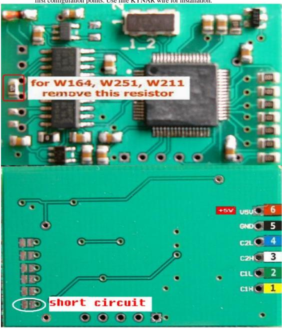
Remove from EZS board SMD part marked with red "X". With short, good isolated wire connect Mercedes CAN filter to EZS board according picture: 1-1 (C1H), 2-2(C1L), 3-3(C2H), 4-4(C2L), 5-5(GND), and 6-6 (+5V).
