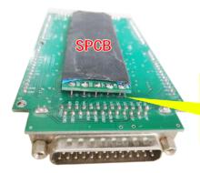
Step1. Remove SPCB Attention: Do not damage the PCB pad
